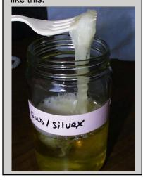
**Transitioning to new AR-FFFs.** - Empty and flush foam tank(s). Do so in cooperation with environmental regulations which may vary by jurisdiction. Discarded concentrate and rinse water will need to be captured, clearly labeled and dispose of in accordance with environmental authority having jurisdiction.
